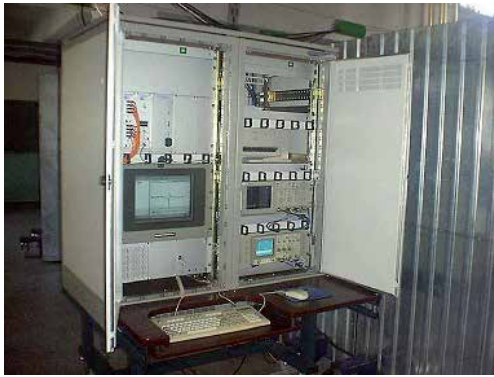
Fig. 4.8. Monitoring and control system for PF-1000 diagnostics in a Faraday cage
