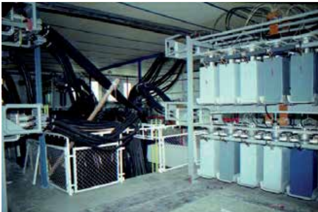
Fig. 4.1. The upper part of the PF-1000 capacitor bank. A view of one of the twelve modules containing 24 capacitors. (SCHOLZ ET AL., 2000)
